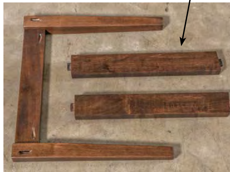
leg assembly glued & pocket-screwed
